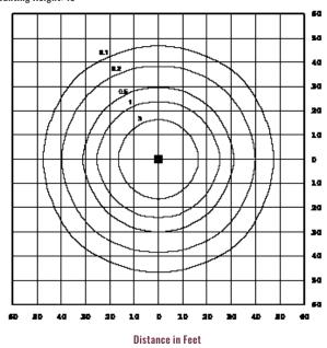
Note: All published photometric testing performed to IES LM-79 standards. Fixture photometry was completed on a single representative fixture. Foot candle levels are noted inside graph.
